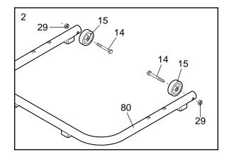
3. With the help of a second person, carefully tip the treadmill onto its left side. Hold the Base (80) against the Right Handrail (6) and the Left Handrail (not shown). **Make sure the Wheels (15) are toward the front of the treadmill as shown.**
